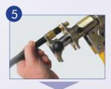
Slide the jointing sleeve towards the fitting. Position the jointing sleeve and the fitting squarely within the jaws of the PSC Compression Tool.
