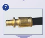
Inspect the joint to ensure the sleeves are drawn all the way to the fitting shoulder and the beveled end of the sleeves is towards the fitting.
